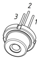
Free-space uncooled TO9 and TO56 canned packages (standard package, AR-coated glass window, PD monitor)
